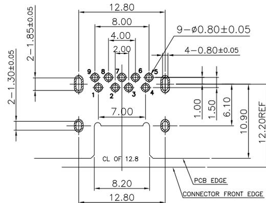
TOLERANCE:  $\pm 0.05$ , THICKNESS: 1.2mm
