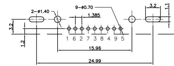
RECOMMENDED P.C.B LAYOUT(PCB THICKNESS: 1.6mm)
